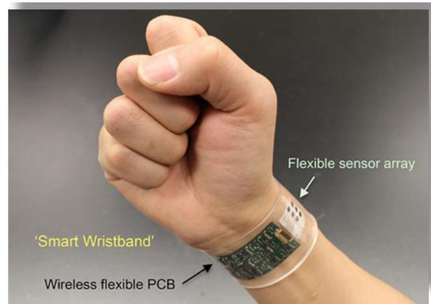
Wearable sweat sensor developed by researchers at UC Berkeley and Stanford.
