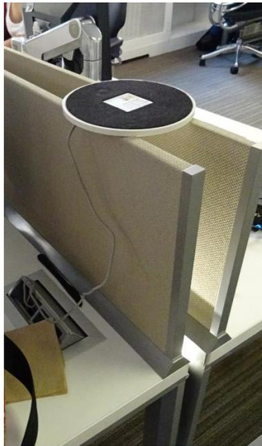
**Figure 5. A sensor-controlled task light annoyed one occupant who turned it upside-down, rather than simply turning it off.**
