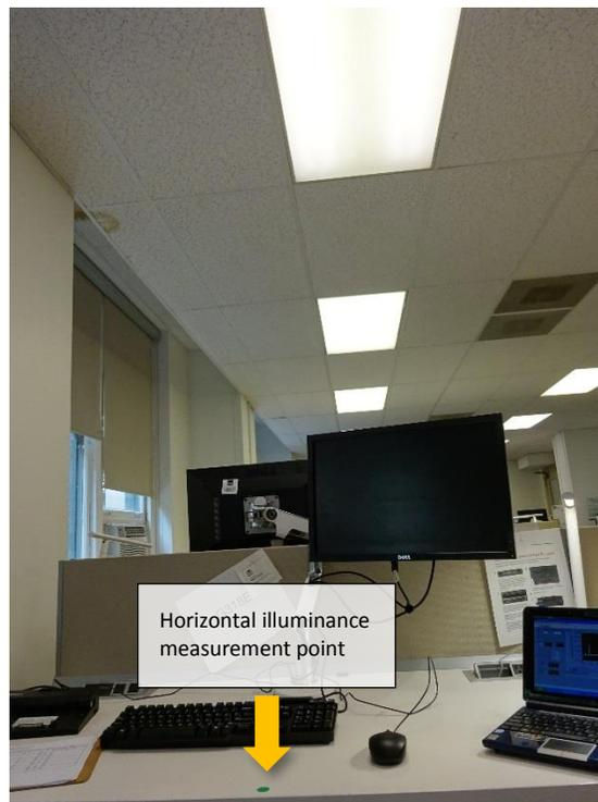
*Figure 2. Typical horizontal measurement points at a row A desk.*
