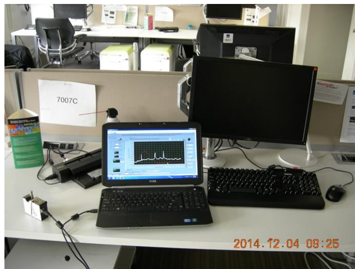
Figure 11. A spectroradiometer taking measurements at desk level.
