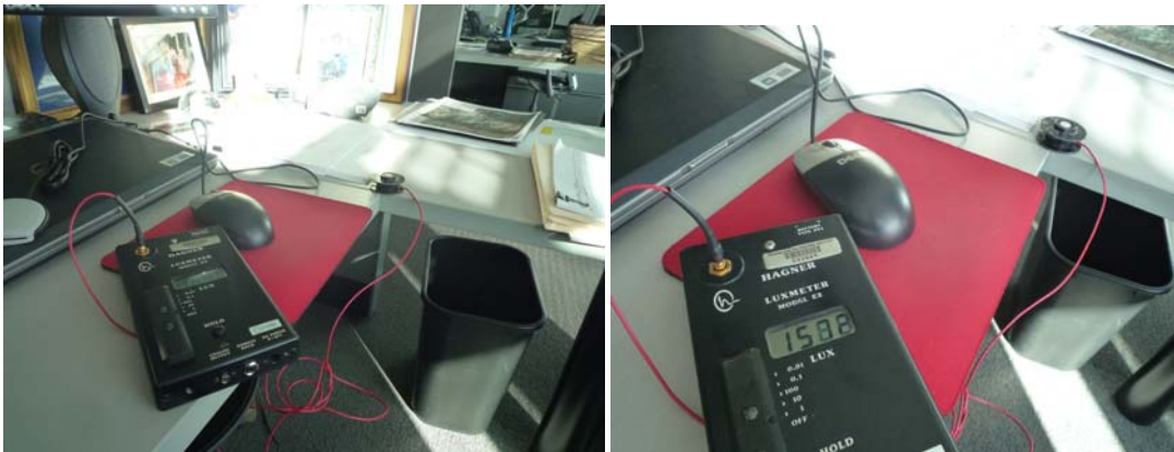
10:30, Desk 361, Illuminance measurement on desk near shaft of sun
