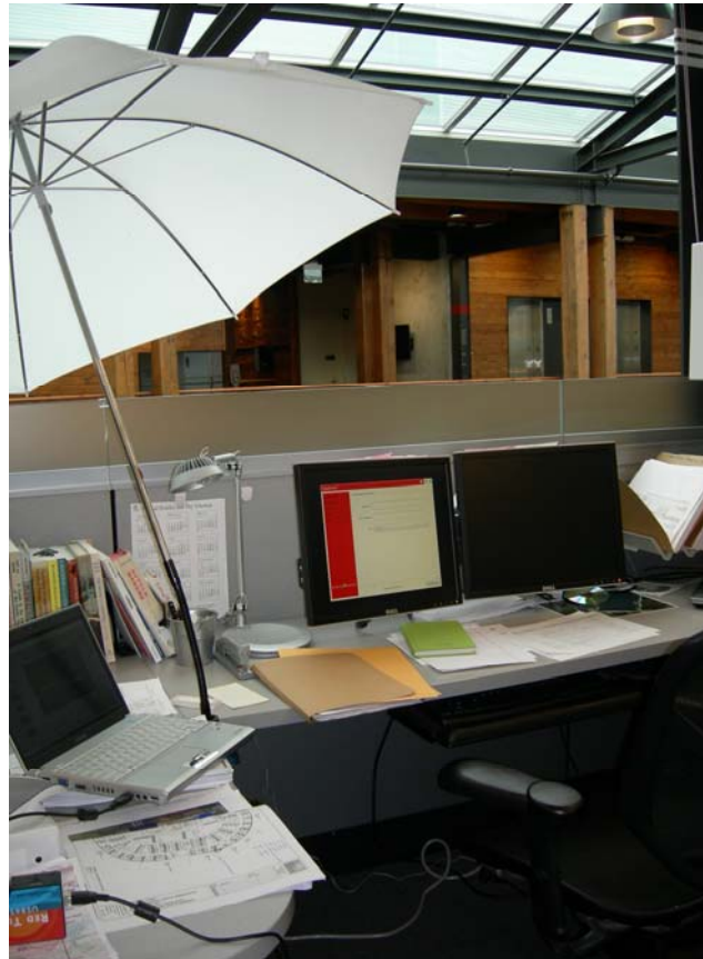
13:29, Desk 616, looking West. Note umbrella and visible skylight. Laptop and Red/Blue device is Spectroradiometer.
