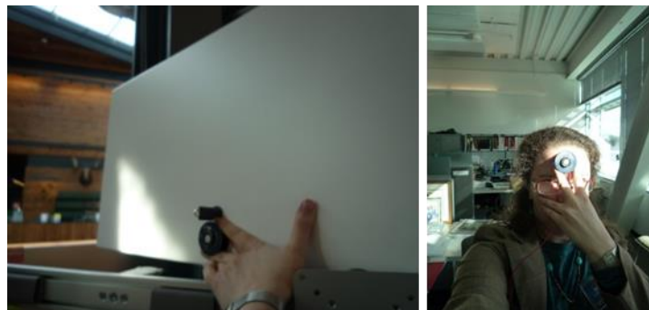
Figure 8. Vertical illuminance measurement examples at cabinet (left) and at the eye (right).
