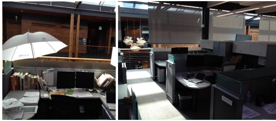
Figure 15. Examples of shading due to atrium skylight. Occupants use golf umbrellas (left) and roll-down shades (right) to diminish glare.
