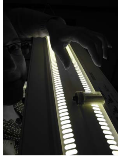
Figure 13. An LRC researcher installs a battery-powered light meter in a luminaire.
