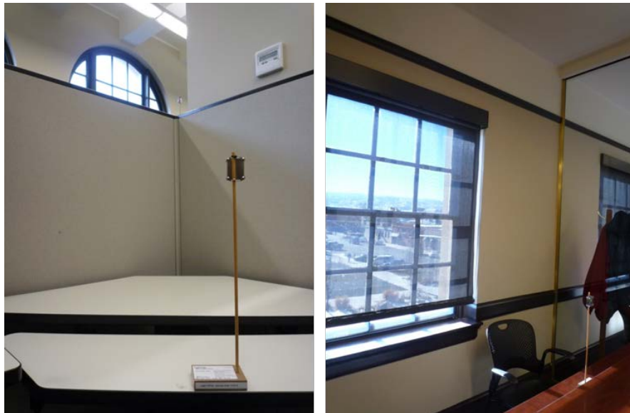
Figure 5. (A, left) A Daysimeter measures circadian light exposure. (B, right) Daylight comes in through an office window.
