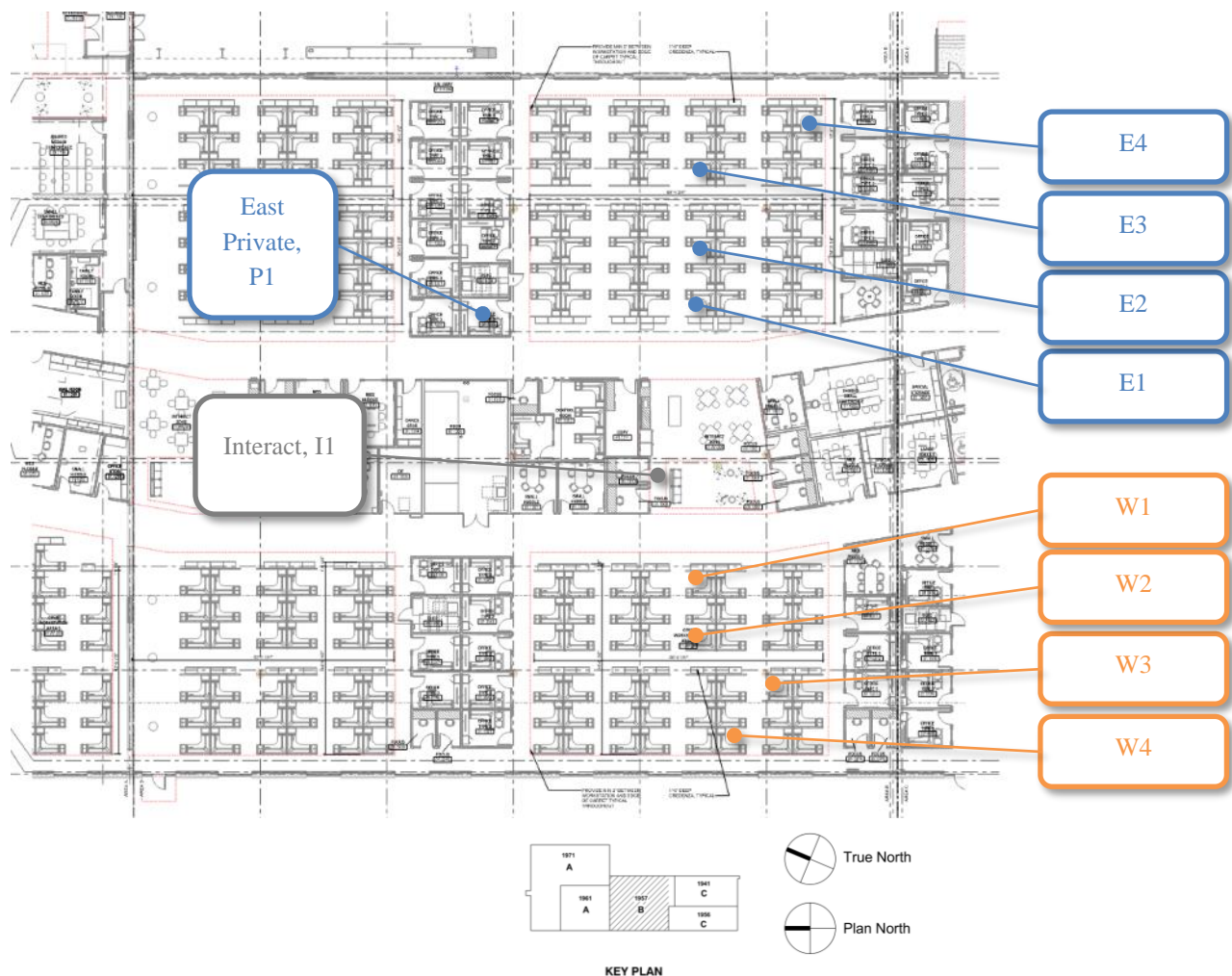
Figure 1. Measurement locations, central section of Building 48.
