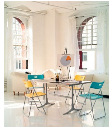
Figure 4. Interior walls of this historic office building are kept light colored to reflect daylight from the large windows.
