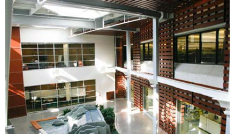
Figure 5. A building atrium with skylights and large exterior windows can provide a circadian “oasis” where employees can go to be exposed to high daylight levels.
