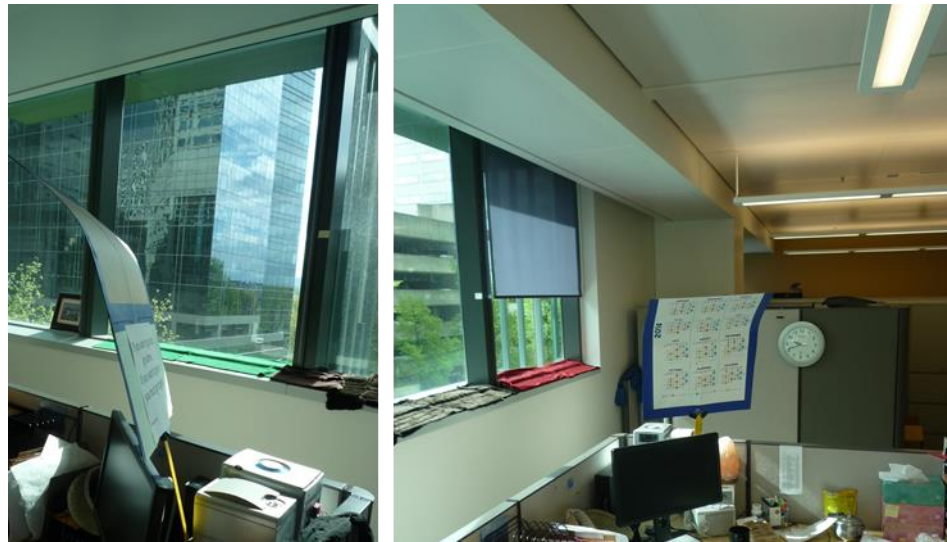
Figure 20. One worker used fabric and cardboard to limit direct and reflected glare.
