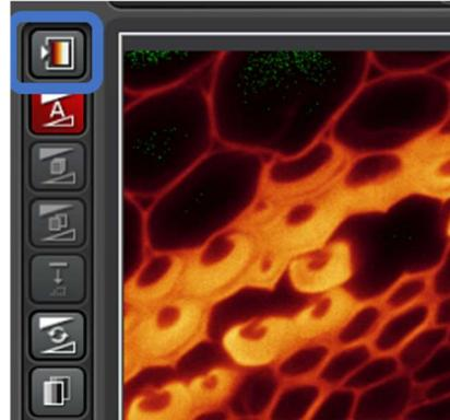
16. Adjust the “Exposure [ms]” (Image) and the LED power (light path) as needed. Consider using *Binning* to improve the *Signal-to-Noise Ratio*.
